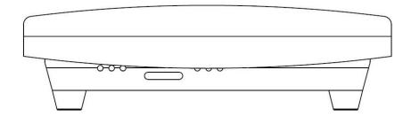
**Power Switch:** The switch is on the left and the red LED is on, which is turn off and charging.
