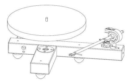
4. Installing the belt: Start with the belt (Part no.6) around the motor pulley, take care the other end clears the centre spindle and rotate the platter (Part no. 1), the belt will track around the platter. We recommend a ½ twist be applied to the belt on the motor pulley:
