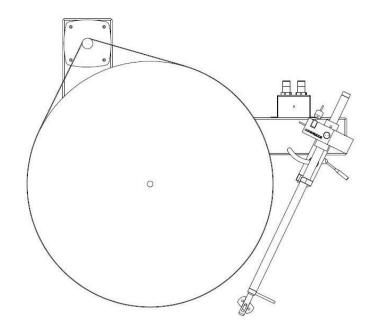
5. There are two grooves on the motor pulley for different speeds. The above groove is for 45 rpm, and the lower groove is for 33.3 rpm. Speed is factory adjusted. If you wish to check the speed place the strobe disc on the platter and using a suitable filament light (Lamp) gently adjust speed potentiometer (Part no. 9) to achieve correct speed.
