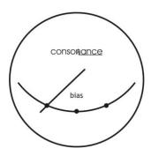
There is a bias indicator of power tubes V1~V8 set on the front side of transformers cover. Note: Normal operating point has been factory set at 55mA, the right point of the indicator. Don't leave the operating point beyond that point, the further right in this case.
