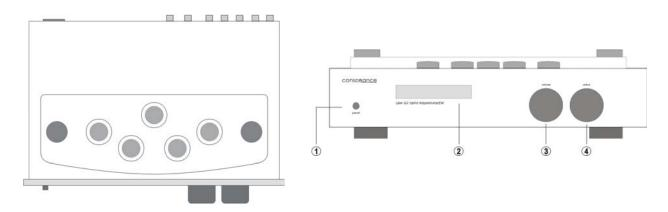
The preamplifier is switched on with the button ① in the left of the front panel. A flashing " -- -- -- blue light in the display ② indicates that power is switched on. By pushing the same button one more time the power is switched off.
