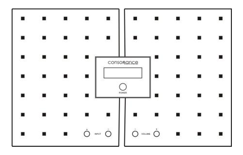
The amplifier is switched on with the button in the middle of the front panel. A red LED in the display, indicates that power is switched on. By pushing the same button one more time the power is switched off.
