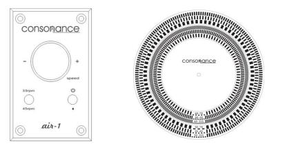
6. Mount the counterweight and the cartridge. Use the stylus guage adjust the cartridge tracking force. Put the protractor on the spindle of turntable. Let the straight line and the edge of the cartridge is parallel. Move the headshell until the tip fall the black spots .Fix the screw on the top of headshell.
