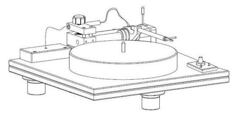
4. Remove the pump from the package. Follow the picture, make sure it use the air tube to connect with the water separator and tonearm. Then turn on pump. If the installation is correct, barometer will show 0.05MPa. Make sure the air bearing move is very smooth.
