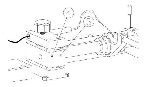
Note2: When the LT-1s is used for a period of time, the inside of the air bearing sleeve will be dirty, which will affect the normal operation. To clean the sleeve, loosen the M6 screw and remove the guide rail. Clean the inside of the sleeve with a wet tissue. After that, re-install the guide rails.
