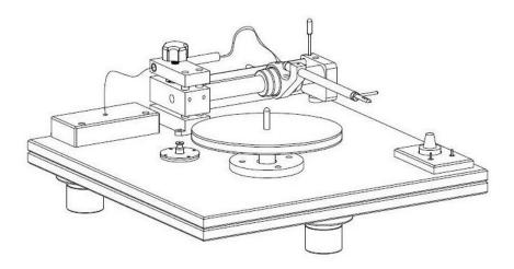
2. Take out one of the drive 'belts' and run it round the motor spindle and then round the driven wheel.
