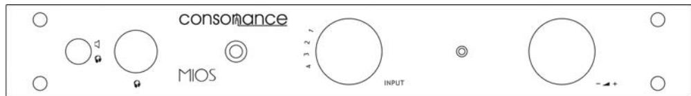
**From left to right are: Mode switch (Headphone or Speaker), Headphone jack , Power indicator,Input selector, IR,Volume control**
