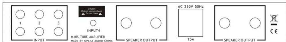
**From left to right are: Input jacks(1,2, 3,4), Speaker connector, Power plug and Fuse, Speaker connector**
