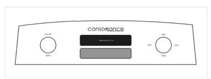
The CD player has only two knobs. The knob on the left hand side of the front panel has 2 function, the right one has 4 function.
