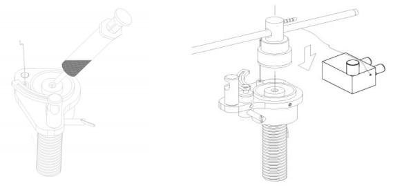
4. In this picture you must secure the tonearm cable connection using the supplied 1.5mm allen wrench. After you place the connection inside the hole in the tonearm base use the allen wrench to tighten the allen screw, located on the side of the base.
