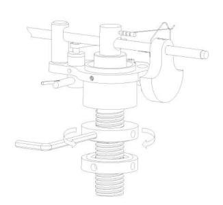
adjustments (first by hand) to reach the proper vertical tracking position then use the 3mm allen wrench to help make a tighter secure fit. After this use the 3mm allen wrench to tighten the screws located around the edge of the threaded washers. Becareful not too tighten these screws too much. Just make sure they are properly secure so that the washers don't become lose over time.
