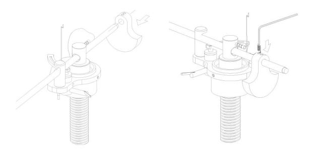
6. Mount your cartridge according to the manufacturer's instructions. Align cartridge for overhang (16mm)and offset angle
