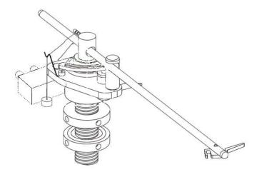
**Note:** The anti-skating force is adjusted according to the mass of the cartridge as follows: T988's downforce: 10-14mN,15-19mN,20mN and bigger(Groove in the stub 1st, 2st, 3st from bearing rings).
