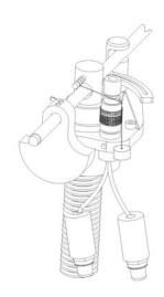
**Note:** The anti-skating force is adjusted according to the mass of the cartridge as follows: T988's downforce: 10-14mN,15-19mN,20mN and bigger(Groove in the stub 1<sup>st</sup>, 2<sup>st</sup>, 3<sup>st</sup> from bearing rings).
